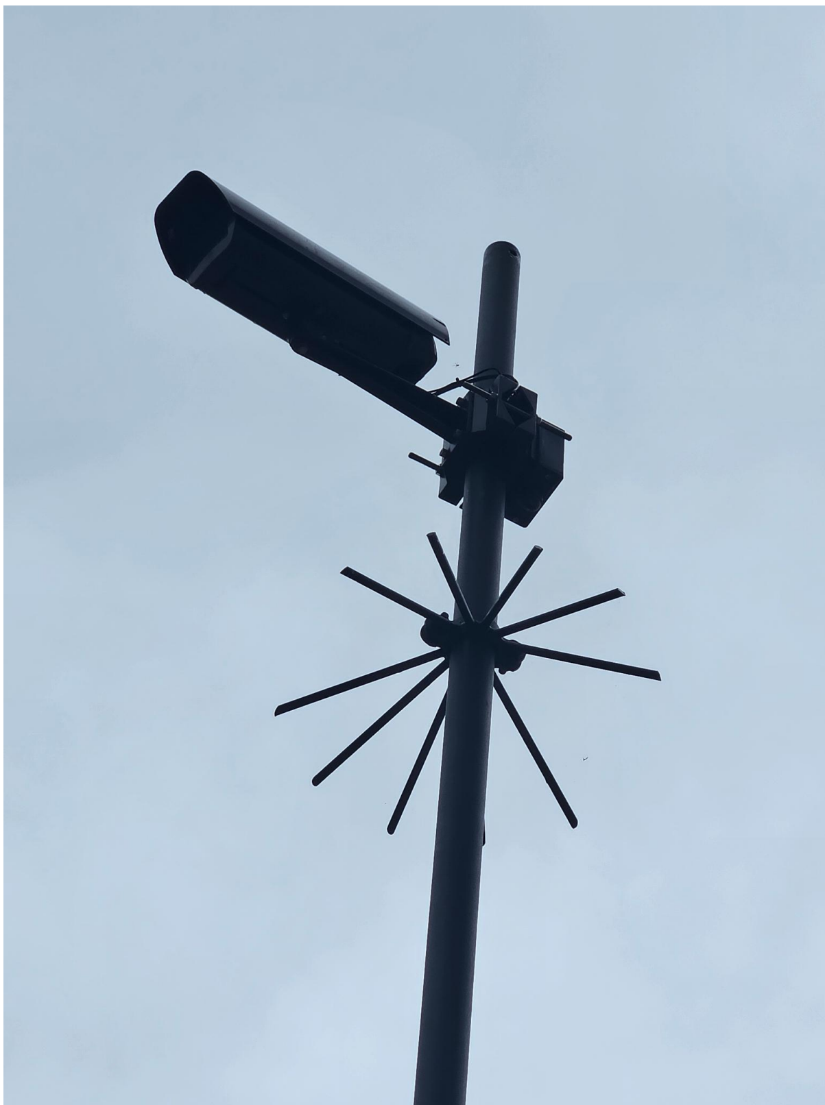
Figure 25: Licence plate recognition camera for the low emission zone — close up
